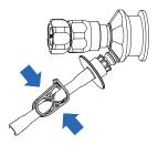
Engage the pinch clamp to seal the Keofitt Sterile Sampling Bag.
