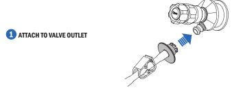
Make sure the sampling valve is pre-sterilised and in its closed position. Attach the Keofitt Sterile Sampling Bag tube fitting to the sampling valve outlet sliding the blue quick coupling ring towards the valve to lock.
